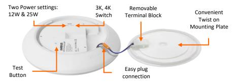
**Emergency function:** When the emergency driver detects the mains power, it will automatically charge the battery. When it detects the absence of mains power, it will turn on the emergency light until the battery is fully discharged or when mains power comes on, it will then stop discharging. After mains power comes on, it will automatically charge the battery normally.
